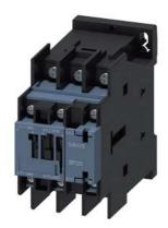
power contactor, AC-3 12 A, 5.5 kW / 400 V 1 NO + 1 NC, 110 V AC, 50 Hz 120 V, 60 Hz, 3-pole Size S0 ring cable lug connection
