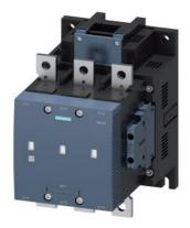
vacuum contactor, AC-3 300 A, 160 kW / 400 V, AC (50-60 Hz) / DC operation 500-550 V AC/DC auxiliary contacts 2 NO + 2 NC 3-pole, frame size S10 busbar connections drive: conventional
