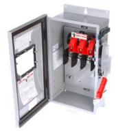
Siemens Low Voltage Circuit Protection Heavy Duty Safety Switches. Type: ENCLOSED, SAFETY SWITCH Std: UL V. Rating: 600V A. Rating: 60A Wattage: 2W No. Of Poles: 3P F. Rating: 60Hz Action: SINGLE THROW Material: 304SS Enclosure: TYPE 12. 2-3 point mounting holes. Insulation: YES O. Cycles: 10000 O. Temperature: (-20F-120F) AMBIENT TEMPERATURE Environmental Conditions: INDUSTRIAL
