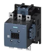
power contactor, AC-3 225 A, 110 kW / 400 V AC (50-60 Hz) / DC operation 96-127 V AC/DC auxiliary contacts 2 NO + 2 NC 3-pole, frame size S10 busbar connections drive: electronic with PLC interface 24 V DC screw terminal
