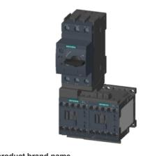
Load feeder fuseless, Reversing duty 400 V AC, Size S00 0.55...0.80 A 230 V AC screw terminal for installation on standard mounting rail (also fulfills type of coordination 1) Type of coordination 2, Iq = 150 kA 1 NC (contactor)
