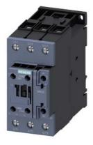
power contactor, AC-3 51 A, 22 kW / 400 V 1 NO + 1 NC, 48 V AC, 50 / 60 Hz, 3-pole, size S2, screw terminal
