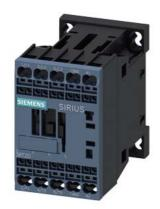
Power contactor, AC-3 9 A, 4 kW / 400 V 1 NO, 42 V AC, 50 / 60 Hz, 3-pole, Size S00 Spring-type terminal
