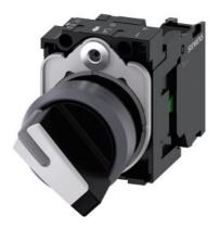
Selector switch, illuminable, 22 mm, round, plastic with metal front ring, white, selector switch, short, 2 switch positions O-I, latching, actuating angle  $90^\circ$ , 10:30h/13:30h, with holder, 1 NO, screw terminal, with laser labeling, upper case and lower case, always upper case at beginning of line
