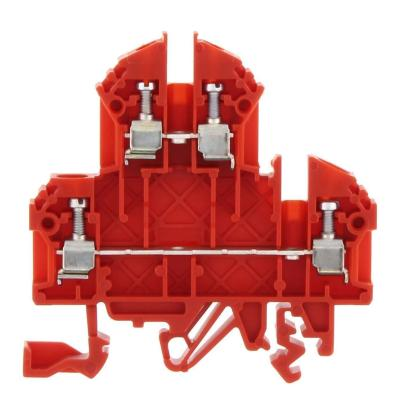
Double-level terminal, Screw connection, Mounting type:Mounting rail TS 35/7.5 and TS 32, Rated cross-section: 2.5 mm², Width: 5 mm, Colour: Red
