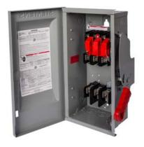
Siemens Low Voltage Circuit Protection Heavy Duty Safety Switches. Type: ENCLOSED, SAFETY SWITCH Std: UL V. Rating: 240V A. Rating: 30 A No. Of Poles: 3P F. Rating: 60Hz Action: SINGLE THROW Material: 304SS Enclosure: TYPE 12. 2-3 point mounting holes. Insulation: YES O. Cycles: 10000 O. Temperature: (-20F-120F) AMBIENT TEMPERATURE Environmental Conditions: INDUSTRIAL
