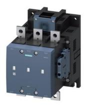
vacuum contactor, AC-3 300 A, 160 kW / 400 V, AC (50-60 Hz) / DC operation 42-48 V AC/DC auxiliary contacts 2 NO + 2 NC 3-pole, frame size S10 busbar connections drive: conventional
