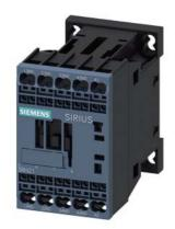
Contactor relay, 3 NO + 1 NC, 24 V AC, 50 / 60 Hz, Size S00, Spring-type terminal
