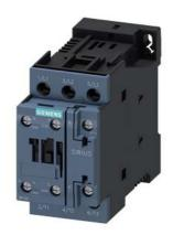
power contactor, AC-3 12 A, 5.5 kW / 400 V 1 NO + 1 NC, AC (50-60 Hz) DC operation 95-130 V AC/DC, 3-pole Size S0, screw terminal
