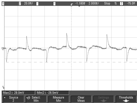
Figure 2 AGQ300 transient response to step in load from 25%~50%~25% ( \Delta I_o/\Delta t = 0.1A/1\mu s )
