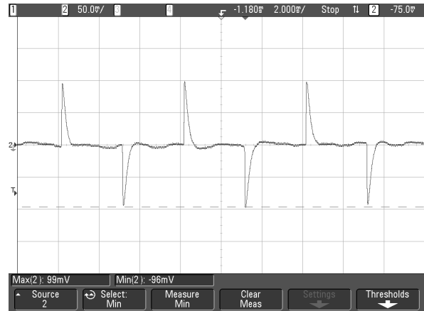
Figure 3 AGQ300 transient response to step in load from 10%~100%~10% ( \Delta I_o/\Delta t = 0.1A/1\mu s )
