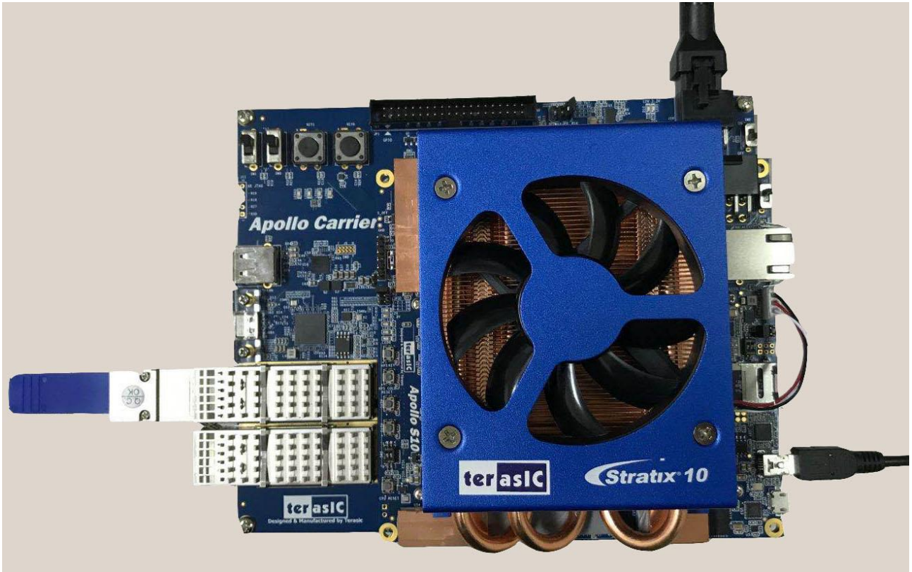
Figure 6-2 QSFP28 Loopback fixtures in the Apollo Develop kit
