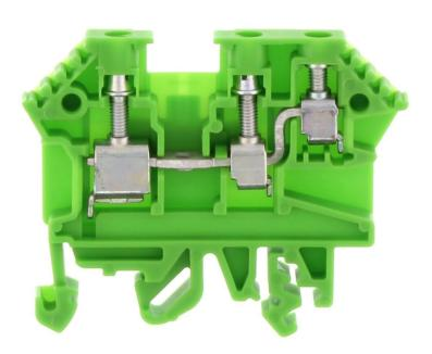
Feed-through terminal, Screw connection, Mounting type:Mounting rail TS 35/7.5 and TS 32, Rated cross-section: 4 mm², Width: 6 mm, Colour: Green
