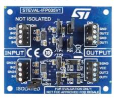
The STEVAL-IFP035V1 evaluation board is designed to help you evaluate circuit protection strategies for factory automation using digital input current limiters between industrial sensor devices and processing units such as programmable logic controllers (PLC). This board embeds two independent CLT03-2Q3 self-powered digital input current limiters.
