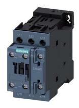
power contactor, AC-3 25 A, 11 kW / 400 V 1 NO + 1 NC, AC (50-60 Hz) DC operation 95-130 V AC/DC, 3-pole, Size S0, screw terminal
