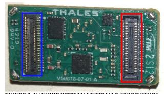
FIGURE 3: NAVCHIP WITH MALE/FEMALE CONNECTORS CALLED OUT
