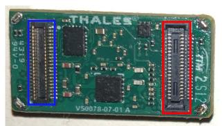
FIGURE 7: NAVCHIP WITH MALE/FEMALE CONNECTORS CALLED OUT
