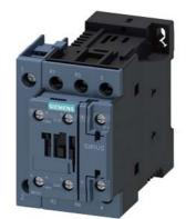
Power contactor, AC-3 25 A, 11 kW / 400 V 2 NO + 2 NC 48 V DC 4-pole size S0 screw terminals 1 NO + 1 NC integrated
