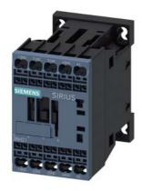
Contactor relay, 2 NO + 2 NC, 480 V AC, 60 Hz, Size S00, Spring-type terminal
