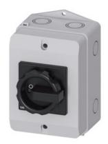
SENTRON, Switch disconnector 3LD, main switch, 3-pole, lu: 32 A, Operating power / at AC-23 A at 400 V: 11.5 kW, molded-plastic encapsulation for metric screw connection, 1 NC, 1 NO, rotary operating mechanism, black
