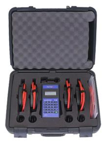
Wide range of fundamental frequency modes for 50Hz, 60Hz, 400Hz, variable frequency systems, and DC to cover all your needs.
