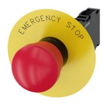
EMERGENCY STOP mushroom-type actuator, 22 mm, round, plastic, red, 40 mm, positive latching, according to EN ISO 13850, pull-to-unlatch mechanism, with yellow backing plate, inscription: EMERGENCY STOP, with holder, 1 NO+1 NC, screw terminal, Z=20-unit packaging
