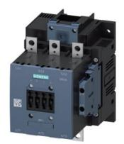
Contactor, AC-1, 275 A/690 V/40  $^\circ$ C, S6, 3-pole, 500-550 V AC/DC, with varistor, 2 NO+2 NC, Connection rail/ screw terminal
