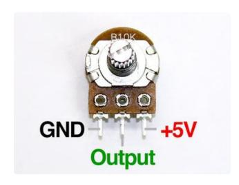
Potentiometers don't care which outer leg is ground or +V, but the choice does affect which direction has increasing output.
