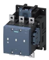
vacuum contactor, AC-3 265 A, 132 kW / 400 V AC (50-60 Hz) / DC operation 96-127 V AC/DC auxiliary contacts 2 NO + 2 NC 3-pole, frame size S10 busbar connections drive: electronic with PLC interface 24 V DC
