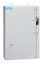
Non-reversing motor starter, Size 2 1/2, Three phase full voltage, Solidstate overload relay, OLR amp range 25-100A, 208VAC 60Hz coil, Combination type, 60A fusible disconnect, 60A/600V fuse clip, Encl NEMA type 4X 304 S-Steel, Water/dust tight noncorrosive, Standard width enclosure
