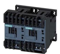
Reversing contactor assembly AC-3,4 kW/400 V,AC24 V,50/60 Hz 3-pole, Size S00 Spring-type terminal electrical and mechanical interlock
