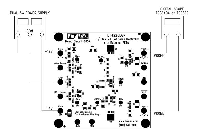
Figure 1. Proper Measurement Equipment Setup
