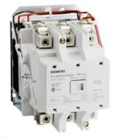
Mechanically held lighting contactor, Contactor amp rating 100A, 0 N.C. / 4 N.O. poles, 24VAC 60HZ coil, Non-combination type, Enclosure NEMA type (open), No enclosure
