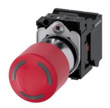
EMERGENCY STOP mushroom pushbutton, illuminable, 22 mm, round, metal, shiny, red, 30 mm, positive latching, according to DIN EN ISO 13850, rotate-to-unlatch, washer for EMERGENCY STOP, yellow, without inscription, with holder, 1 NC, 1 NC, LED module 24 V red, spring-loaded terminal, front plate mounting
