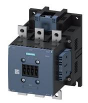
power contactor, AC-3 300 A, 160 kW / 400 V, AC (50-60 Hz) / DC operation 21-27 AC/DC, 3 V auxiliary contacts 2 NO + 2 NC 3-pole, frame size S10 busbar connections drive: electronic with PLC interface 24 V DC spring-loaded terminal
