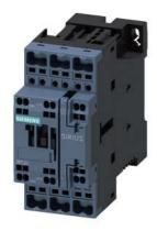
power contactor, AC-3 17 A, 7.5 kW / 400 V 1 NO + 1 NC, 110 V DC, 3-pole, Size S0 Spring-type terminal
