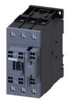
power contactor, AC-3 51 A, 22 kW / 400 V 1 NO + 1 NC, 220 V AC 50 / 60 Hz, 3-pole, size S2, spring-loaded terminal
