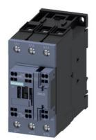
power contactor, AC-3 51 A, 22 kW / 400 V 1 NO + 1 NC, 175-280 V AC/DC with varistor, 3-pole, size S2, spring-loaded terminal
