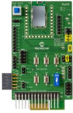
This board enables development with the RN4870 BLE module. The board includes a sensor daughter board for experimentation with on-board light and temperature sensing, a potentiometer, a pushbutton switch and LEDs. The board can be interfaced via USB and any PC terminal program, or over the PICtail interface connected to one of
