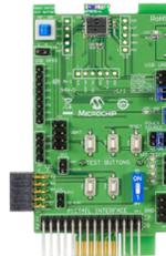
This board enables development with the small form factor RN4871 BLE module. The board can be interfaced via USB and any PC terminal program, or over the PICtail interface connected to one of Microchip's microcontroller development boards such as the Explorer 16 Development Board.
