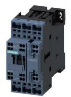
Power contactor, AC-3 32 A, 15 kW / 400 V 1 NO + 1 NC, AC (50-60 Hz) / DC 200- 280 V AC / DC 3-pole, Size S0, Spring-type terminals
