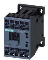
power contactor, AC-3 7 A, 3 kW / 400 V 1 NO, 24 V DC 0.7-1.25\* US, 3-pole, size S00, spring-type terminal suitable for PLC outputs not expandable with auxiliary switch
