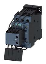
Capacitor contactor, AC-6b 20 kVAr, / 400 V 1 NO + 2 NC, 110 V DC 3-pole, Size S0 screw terminal
