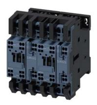
Reversing contactor assembly AC-3, 5.5 kW/400 V 110 V AC 50 Hz/120 V 60 Hz, 3-pole Size S0, Spring-type terminal electrical and mechanical interlock
