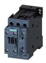
Power contactor, AC-3 32 A, 15 kW / 400 V 1 NO + 1 NC, 24 V DC 3-pole, size S0 screw terminals Upright mounting position
