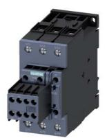
Power contactor, AC-3 65 A, 30 kW / 400 V 2 NO + 2 NC, 220 V AC 50/60 Hz, 3-pole Size S2, screw terminals
