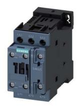
power contactor, AC-3 17 A, 7.5 kW / 400 V 1 NO + 1 NC, AC (50-60 Hz) DC operation 200-280 V AC/DC 3-pole, Size S0, screw terminal
