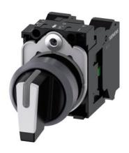
Selector switch, illuminable, 22 mm, round, plastic with metal front ring, white, selector switch, short, 3 switch positions I>O<II, momentary contact type, actuating angle 2x45°, 10:30h/12h/13:30h, with holder, 1 NO, 1 NO, spring-type terminal, with laser labeling, upper case and lower case, always upper case at beginning of line
