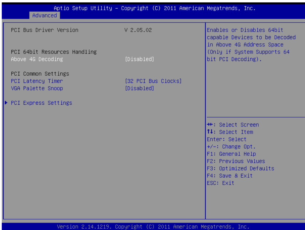
Figure 3.5 PCI Subsystem Settings
