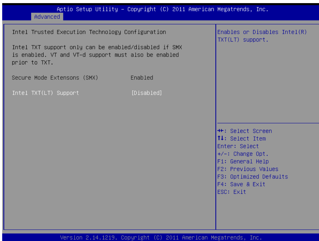
Figure 3.12 Intel Trusted Execution Technology Configuration
