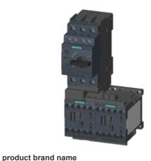
Fuseless motor starter Reversing operation 600VAC Size S00 2.2-3.2A 24V DC screw connection For screw mounting Or 35 mm rail-mounting Type of coordination 2 IQ = 150 KA Also full fills type Of coordination 1 1NO+1NC (MSP) 1NC (per contactor)
