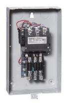
Non-reversing motor starter, Size 2 1/2, Three phase full voltage, Amb compensate bimetal OLrelay Contactor amp rating 60Amp 550/575 600 50/60HZ coil, Non-combination type, Enclosure type 1, Indoor general purpose use
