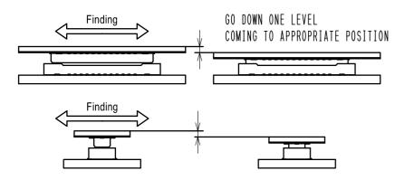
(2) WHEN GUIDING, THE CONNECTORS ARE ALIGNED PARALLEL TO EACH OTHER, WITH LONGITUDINAL AND LATERAL MOVEMENTS RESTRICTED. MATE THEM PROPERLY BY APPLYING FORCE IN THIS CONDITION.
