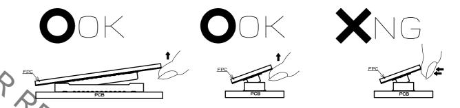
FPC IS NOT RIGID, THE CONNECTOR CAN BE BROKEN. PLEASE CHECK THE ACTION OF THE FPC TO BE USED REPEATERLY AT THE TIME OF TRIAL PRODUCTION. BE CAREFUL TO UN-MATE THEM FROM THE PITCH DIRECTION, THE CORNER CAN ALSO RISK TO PUTTING STRESS ON CONTACTS.
