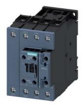
Contactor, AC-1, 110 A/400 V/40  $^{\circ}\text{C},$  S2, 4-pole, 20-33 V AC/DC, with varistor, 1 NO+1 NC, screw terminal
